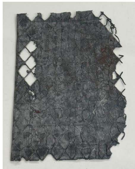
Shedding of active material is the #1 killer of lead/acid batteries
