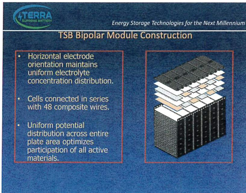
The slide below shows TSB Group 31 Core with terminals cast onto monopolar plates at each end of the core. Total number of composite conductors attached to terminals is ~1500. Ampacity of each composite conductor is ~5 Amps, limiting total current to ~7,500 Amps. The second slide below illustrates how core, terminal and container are assembled to maintain horizontal orientation of electrodes in final assembly
